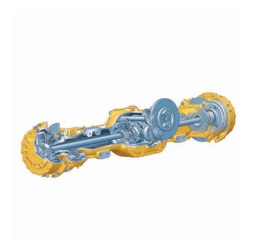
**Front Suspension.** Three-point front suspension oscillates  $\pm 6^{\circ}$  to provide a smooth ride, allowing the 730 to travel at speed over rough terrain and softening impact loads on structures and components.
